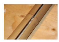
Broker). Typically, the rod maker introduces a "check split" into each culm to allow for expansion and contraction. which reduces the likelihood of producing elsewhere in the culm during storage.
